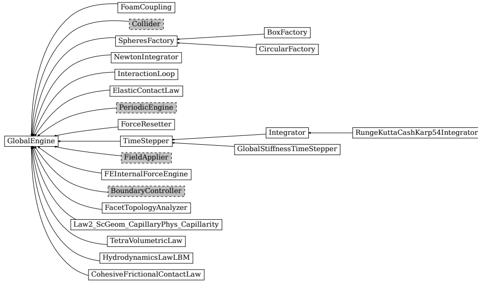
Fig. 25: Inheritance graph of GlobalEngine, gray dashed classes are discussed in their own sections: Collider , PeriodicEngine , FieldApplier , BoundaryController . See also: BoxFactory , CircularFactory , CohesiveFrictionalContactLaw , ElasticContactLaw , FEInternalForceEngine , FacetTopologyAnalyzer , FoamCoupling , ForceResetter , GlobalStiffnessTimeStepper , HydrodynamicsLawLBM , Integrator , InteractionLoop , Law2_ScGeom_CapillaryPhys_Capillarity , NewtonIntegrator , RungeKuttaCashKarp54Integrator , SpheresFactory , TetraVolumetricLaw , TimeStepper .
